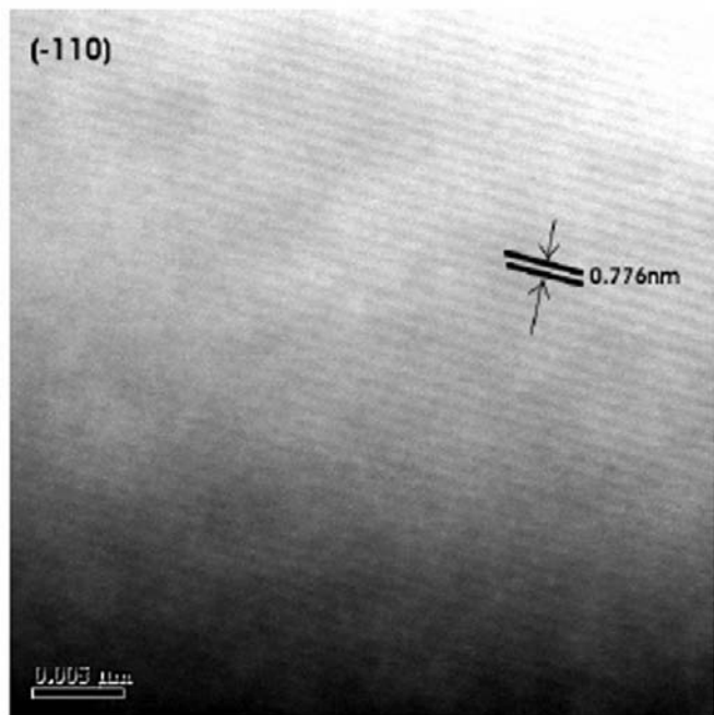
Figure 8 TEM Z-contrast image along the [\bar{1}10] direction. The bright lines indicate rows of Sm atoms.
